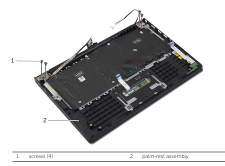
**5** Open the palm-rest assembly as far as possible to release the display hinge from the palm-rest assembly.
