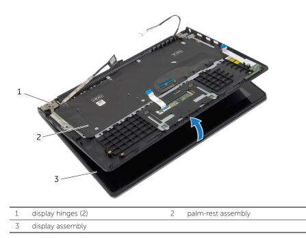
6 Lift the palm-rest assembly away from the display assembly.
