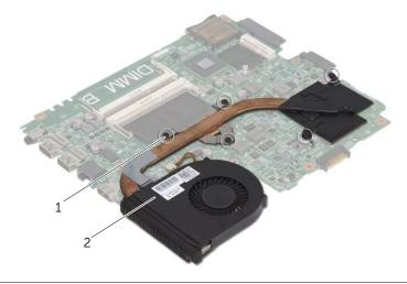
1 captive screws (5) 2 thermal-cooling assembly
