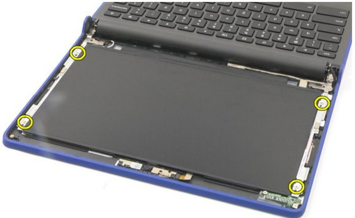
2. Lift the LCD up and rotate it 180 degrees.
