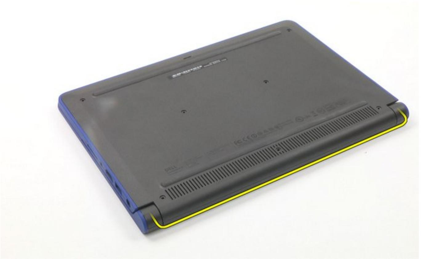
3. Lift up and remove the bottom cover.
