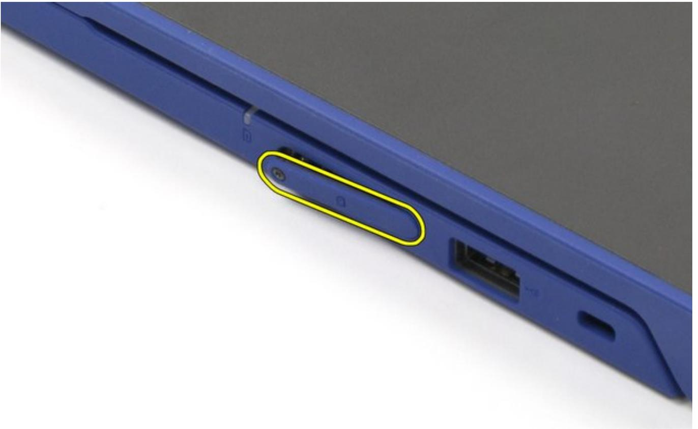
3. Use the push pin to eject the sim card.
