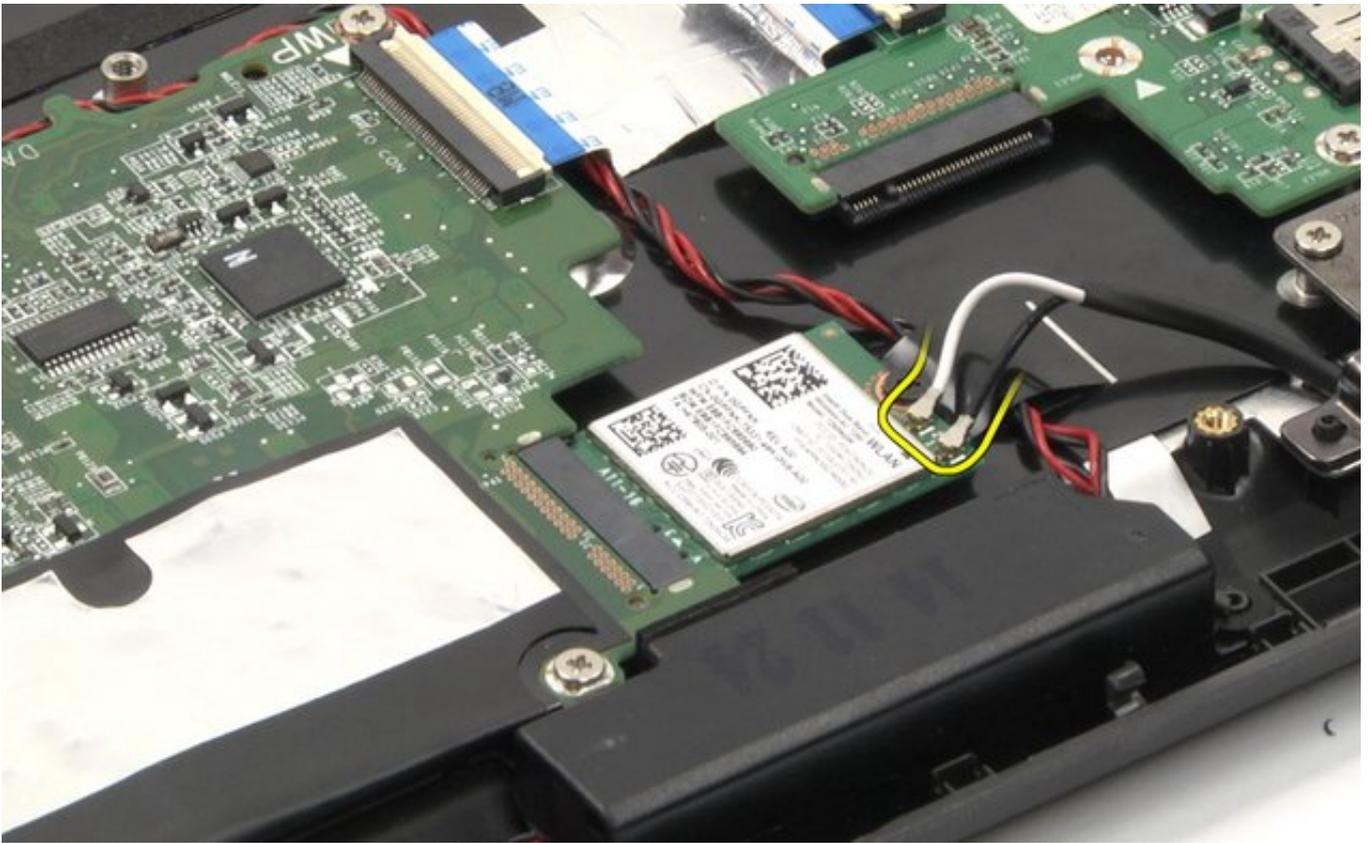
3. Remove one screw securing the WLAN card.
