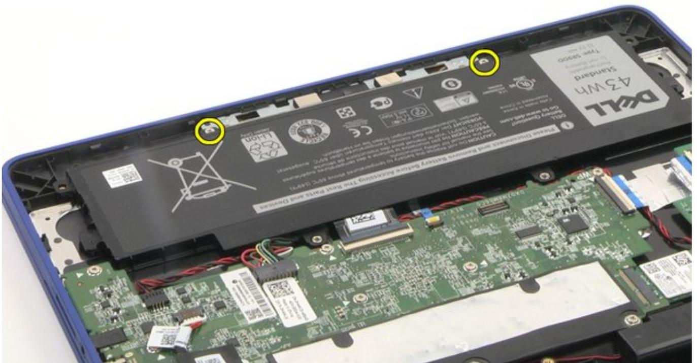
2. Slowly pull the battery to disconnect the battery cable from system board, and remove the battery from the system board.
