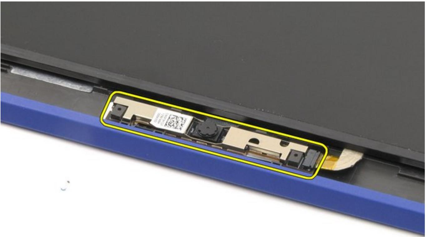
2. Disconnect the camera cable and remove the camera.
