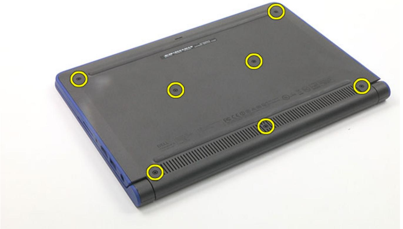
2. Pry up the bottom cover carefully, starting from the top corners.
