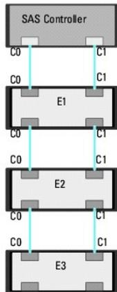
If the communication channel between the connector and the first enclosure is lost, the redundant path configuration itself is lost. In this case, the health of the logical connector is displayed as critical. Navigate to the **Information/Configuration** subtab of the logical connector to view details of the "[Path Health](#)." See the table below for a brief outline of this scenario.
