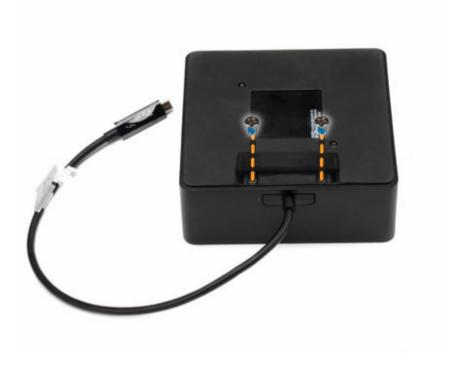
4. Lift and remove the metal cable bracket.
