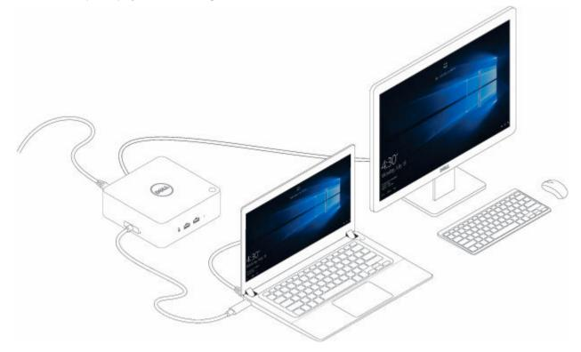
NOTE: Computers requiring more than 130 W power input must also be connected to their U own power adapter for charging and operating at full performance.
