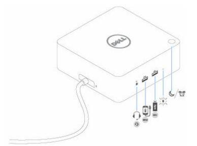
Figure 1. Identifying Parts and Features - Front
