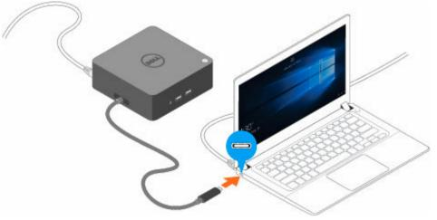
Figure 4. Connecting the Thunderbolt 3 (Type-C) connector
