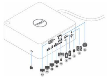
Figure 2. Identifying Parts and Features - Back
