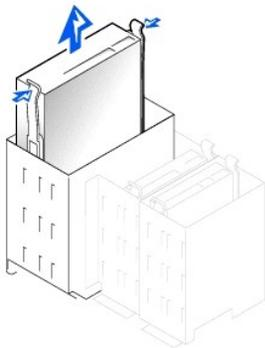
6. Slide the drive upward and remove it from the computer.
