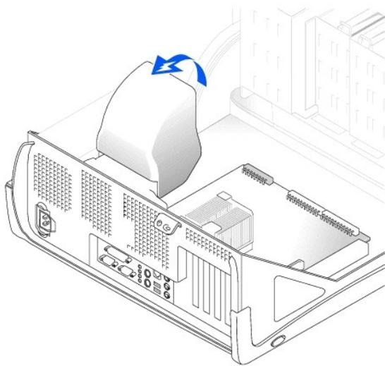
4. Remove the securing clips to remove the heat sink/blower assembly.
