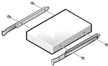
7. Attach the bracket to the new drive by aligning the screw holes on the drive with the screw holes on the rails and tightening all four screws.
