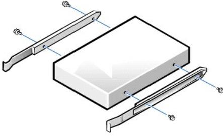
8. Attach the bracket rails to the new hard drive by aligning the four screw holes of the drive and bracket and then inserting and tightening the screws that came with your upgrade kit.
