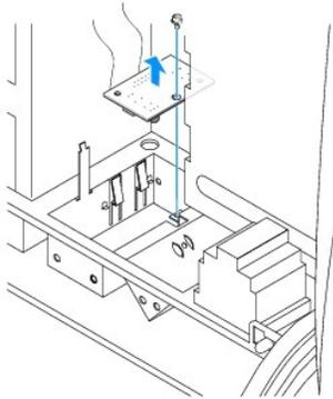
2. Using an 8-inch #2 Phillips screwdriver, remove the screw that secures the control panel to the computer, and lift the panel away from the computer.
