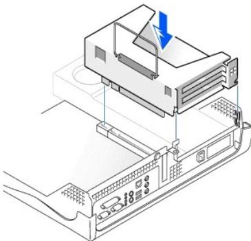
2. Make sure that the riser board is fully seated in the connector on the system board.
