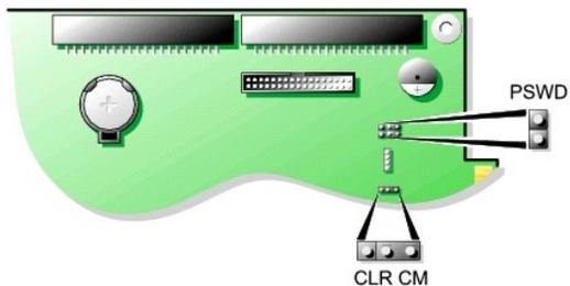
**NOTICE:** Before changing a jumper setting, verify that the standby power light on the system board has turned off. Otherwise, damage to your computer or unpredictable results may occur. To locate this light, see "[System Board Components](#)."
