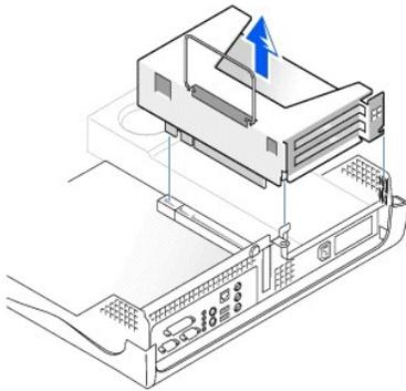
3. Gently pull on the handle and lift the expansion-card cage away from the computer.
