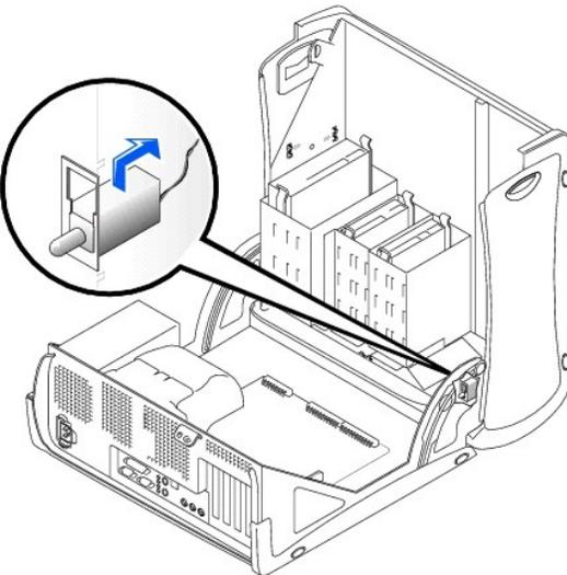
2. Disconnect the chassis intrusion switch cable connector from the control panel on the front of the computer.
