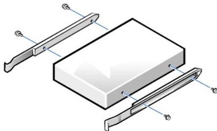
8. Attach the bracket to the new drive by aligning the screw holes on the drive with the screw holes on the bracket rails and tightening all four screws.
