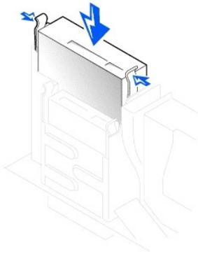
10. Reinstall the removable media drive and bracket assembly by gently sliding the bracket into place until the tabs securely click into position.
