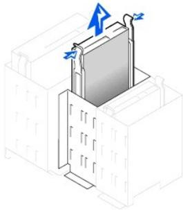
6. If the replacement drive does not have the bracket rails attached, remove the rails from the old drive by removing the two screws that secure each rail to the drive.
