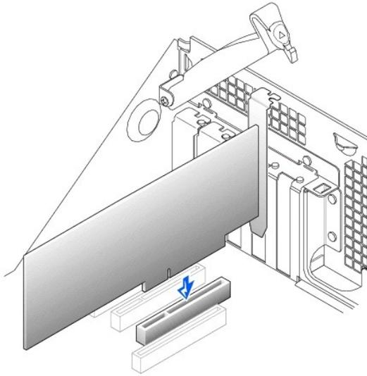
5. If you are installing a new expansion card, remove the filler bracket for an empty card-slot opening. Then continue with step 6.
