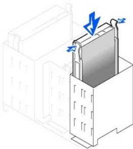
9. Connect a power cable to the power cable connector on the back of the drive, and connect the hard-drive data cable to the hard-drive data cable connector on the drive.
