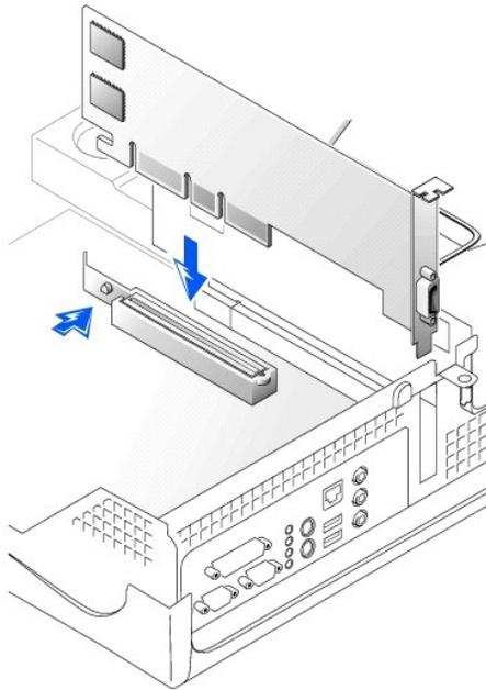
5. Release the AGP card clip lever, ensuring that the tab on the AGP card clip lever fits into the notch on the front end of the AGP card.
