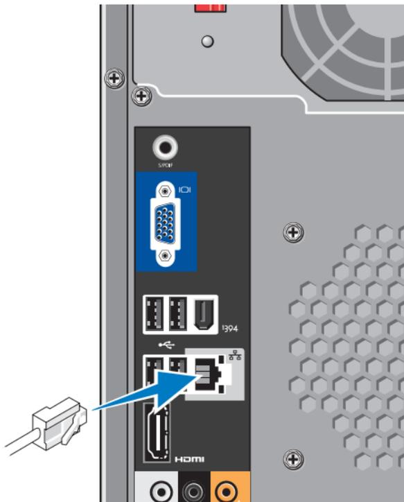
A network connection is not required to complete your computer setup, but if you have an existing network or Internet connection that uses a cable connection (such as a home cable modem or Ethernet jack), you can connect it now. Use only an Ethernet cable (RJ45 connector). Do not plug a telephone cable (RJ11 connector) into the network connector.
