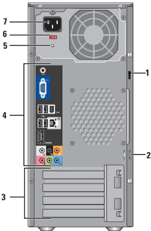
**1 Security cable slot** — Connects to a lock for a security cable used as an anti-theft device.
