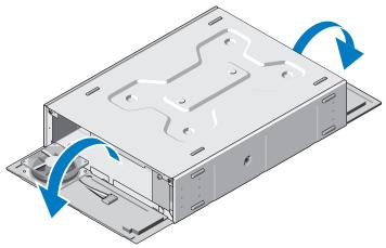
Remove the screws and open the top cover.
