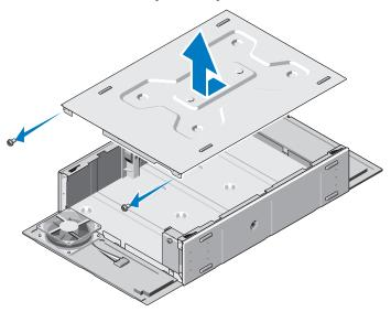
Loosen the screw and remove the cable cover.
