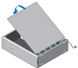
Remove the front-panel and back-panel screws from the IP51 kit.
