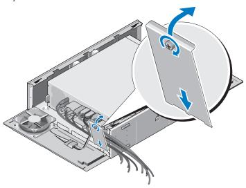
Replace the top cover and replace the screws.
