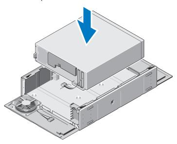
11 Fix the screws (supplied with IP51 kit) on the sides of the IP51 kit.
