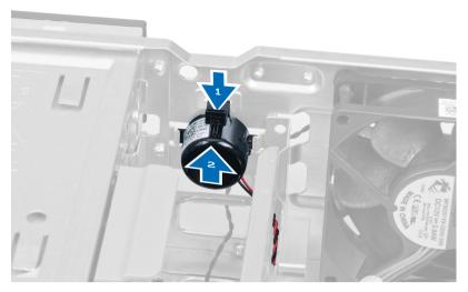
4. Press down the speaker-securing tab and slide the speaker upwards to remove it.
