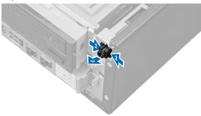
5. Slide the power-switch cable out through the front of the computer.
