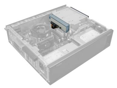
3. Remove the data cable and power cable from the back of the optical drive.
