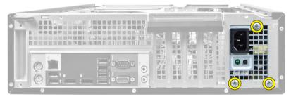
**9.** Push in on the blue release tab beside the power supply, and slide the power supply towards the front of the computer.
