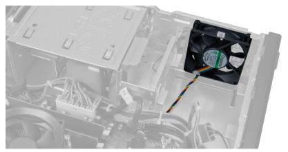
3. Press the plastic clip to release the system-fan cable from the system board.
