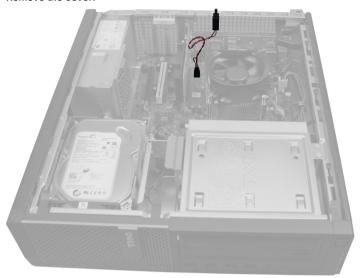
3. Press the clip inwards to release and gently pull the intrusion cable from system board.
