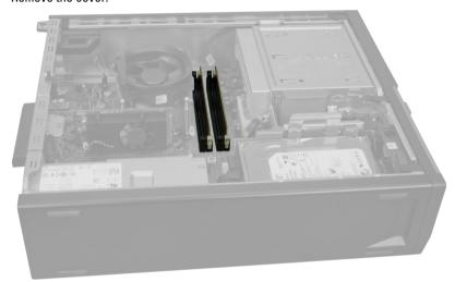
Press down on the memory retaining tabs on each side of the memory modules, and lift the memory modules out of the connectors on the system board.
