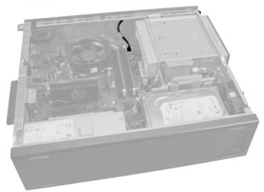
3. Press in and lift to release the power-switch cable from the system board.
