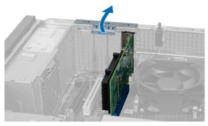
4. Press the release lever away from the expansion card and ease the card up and out of its connector.
