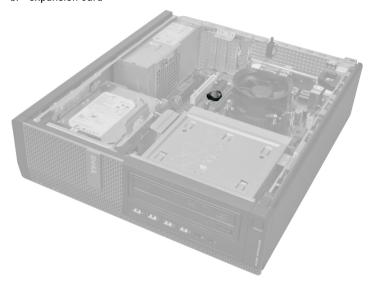
Carefully press the release latch away from the battery. The battery pops out from the socket, lift the coin-cell battery out of the computer.
