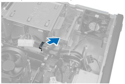
**8.** Pry and remove the system fan away from the four grommets securing it to the computer.
