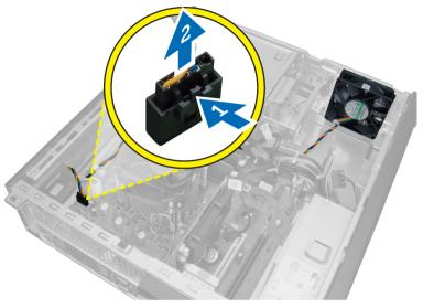
4. Unthread the system-fan cable from the chassis clip.
