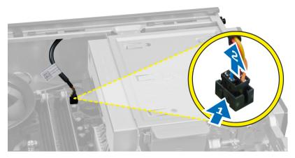
**4.** Press the clips on both sides of the power switch to release it from the chassis and pull the power switch out of the computer.
