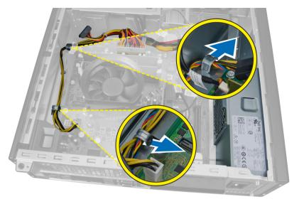
5. Press and lift the 24-pin cable to disconnect it from the system board.
