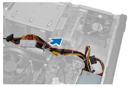
7. Unthread the power supply cables from the chassis clip.
