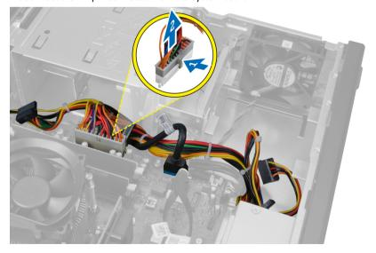
4. Unthread and release the power cable and I/O cable from the chassis clip.
