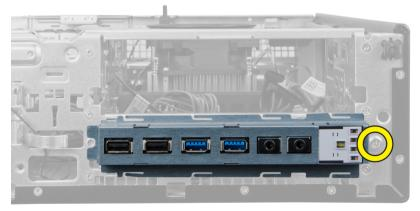
Slide the I/O panel towards the left of the computer to release it and pull the I/O panel along with its cable out of the computer.
