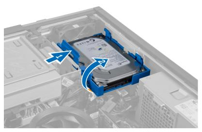
5. Flex the hard drive bracket and then remove the hard drive from the bracket.
