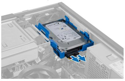
4. Press the blue securing bracket inward and lift the hard drive bracket out of the bay in an angle.
