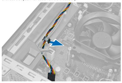
5. Release the system fan cables from the chassis clip.
