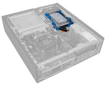
3. Remove the data cable and the power cable from the back of the hard drive.
