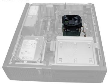
3. Press the plastic clip and pull the heat-sink cable from the system board.
