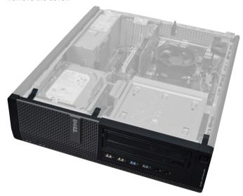
3. Gently pry the front panel retention clips away from the chassis located at the side edge of front bezel.
