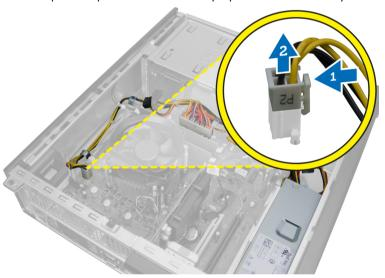
4. Unthread the power cable from the chassis clips.
