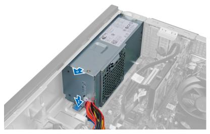
10. Lift the power supply out of the computer.
