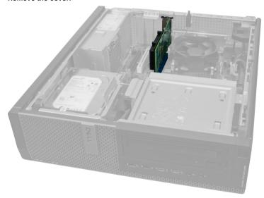
$\textbf{3.} \quad \text{Lift the release tab on the card-retention latch upward.}$
