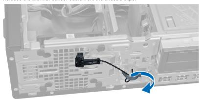
5. Gently press the tabs from both sides to release and remove the thermal sensor away from the chassis.
