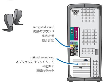
If your integrated sound connectors are covered by a cap, connect your speakers to the optional sound card connectors. Do not remove the cap.
