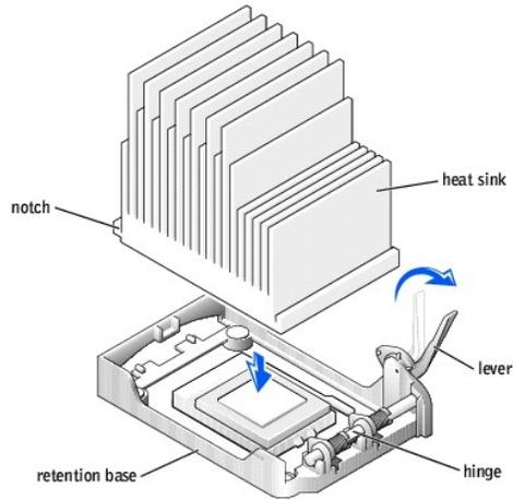
7. Raise the retention lever and press until the heat sink is secured. You will feel the lever pause once it is at a 90-degree angle. Keep pressing the lever another 30 degrees, ensuring that it is in the locked position.
