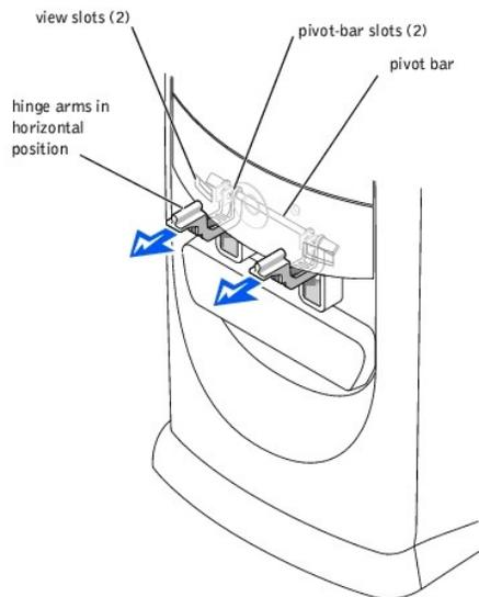
👉 **NOTICE:** Using excessive force to pull the hinge arms into place may damage the arms or the front panel.
