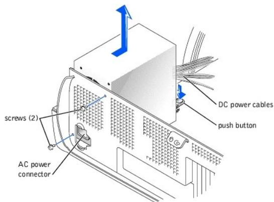
Note the routing of the DC power cables underneath the tabs in the computer frame as you remove them from the system board and drives. It is important to route these cables properly when you replace them to prevent them from being pinched or crimped.
