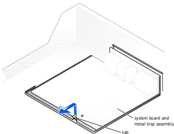
➡ **NOTICE:** The system board and the metal tray are attached and are removed as one piece.
