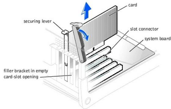
**HINT:** Installing filler brackets over empty card-slot openings is necessary to maintain Federal Communications Commission (FCC) certification of the computer. The brackets also keep dust and dirt out of your computer.
