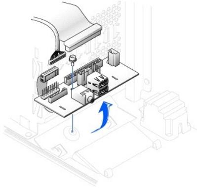
6. Remove all cables that are connected to the front I/O panel.
