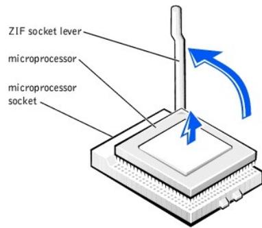
11. Remove the microprocessor from the socket.
