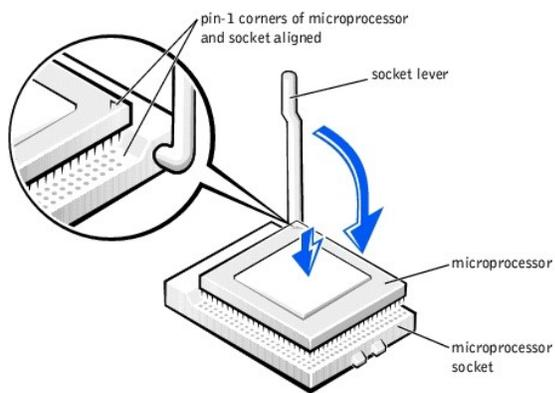
➔ **NOTICE:** The microprocessor pins are delicate. To avoid damage, ensure that the microprocessor aligns properly with the socket, and do not use excessive force when installing the processor.
