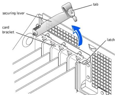
7. To remove the card, grasp the card by the top corners and lift it out.
