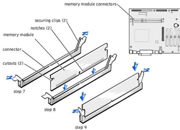
8. Align the notches on the bottom of the module with the crossbars in the connector.
