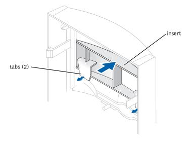
7 Reach inside the computer and push the metal plate towards you so that it snaps off of the computer or insert a small screwdriver inside one of the holes on the front of the metal plate and pry it towards you until it snaps off.
