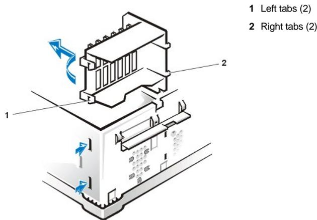
To remove the expansion-card guide, perform the following steps:
