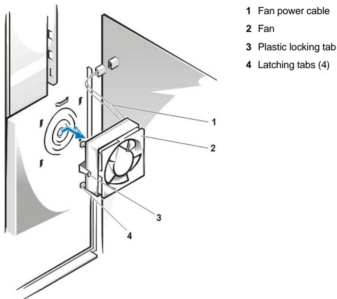
To remove a microprocessor cooling fan, perform the following steps.
