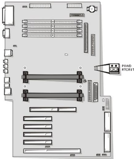
Jumpers are small blocks on a circuit board with two or more pins emerging from them. Plastic plugs containing a wire fit down over the pins. The wire connects the pins and creates a circuit.
