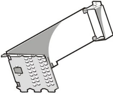
Figure 21 shows the AGP card extension that occludes PCI slots 1 and 2.
