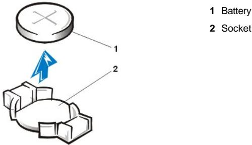
**⚠ CAUTION:** There is a danger of the new battery exploding if it is incorrectly installed. Replace the battery only with the same or equivalent type recommended by the manufacturer. Discard used batteries according to the manufacturer's instructions.
