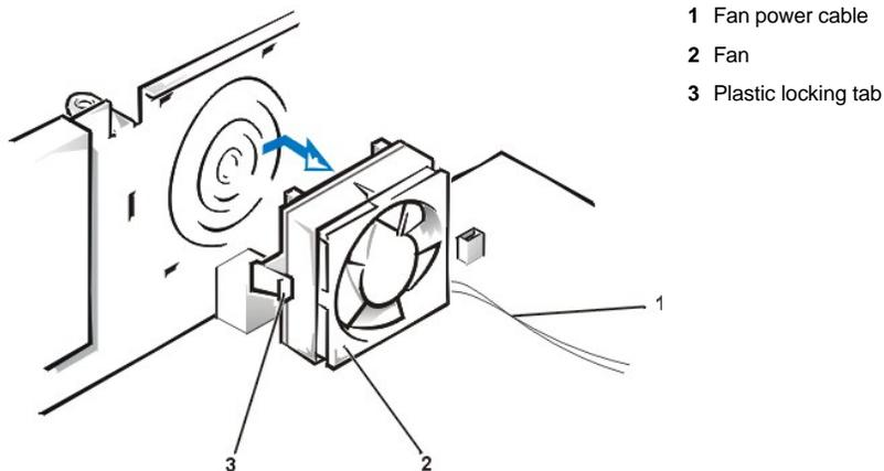
To remove the cooling fan, perform the following steps.
