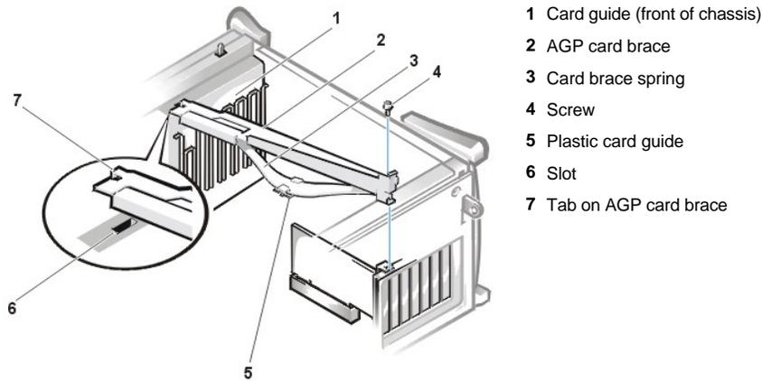
3. Slide the card brace forward until it disengages from the slot in the card guide, then rotate the brace up and lift it away from the chassis.
