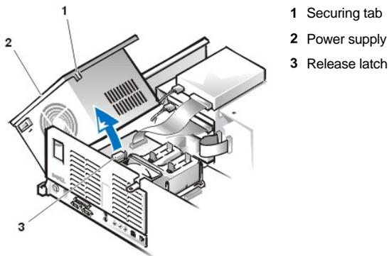
3. Free the power supply by pressing the securing tab labeled "RELEASE" and rotate it upward to a vertical position. See [Figure 20](#).
