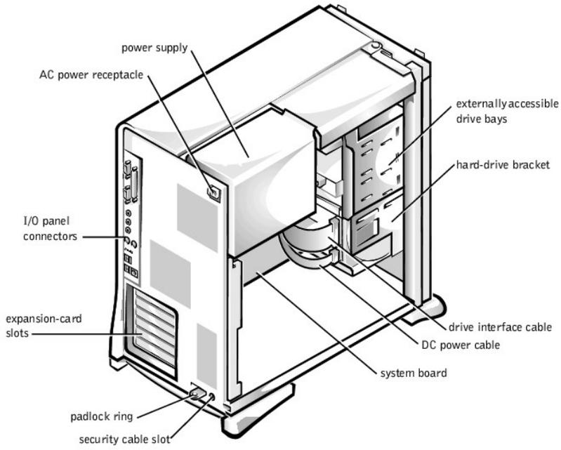
**NOTE:** Before you remove the cover from the mini tower chassis, you must first slide the outer padlock ring to the left to unlock the cover release mechanism. See "[Cover Release Mechanism \(Mini Tower Chassis\)](#)."
