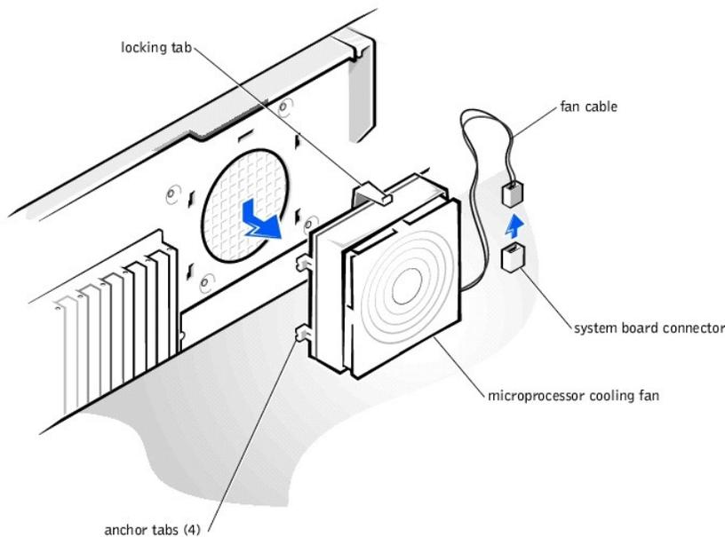
6. Lift the fan out of the chassis.
