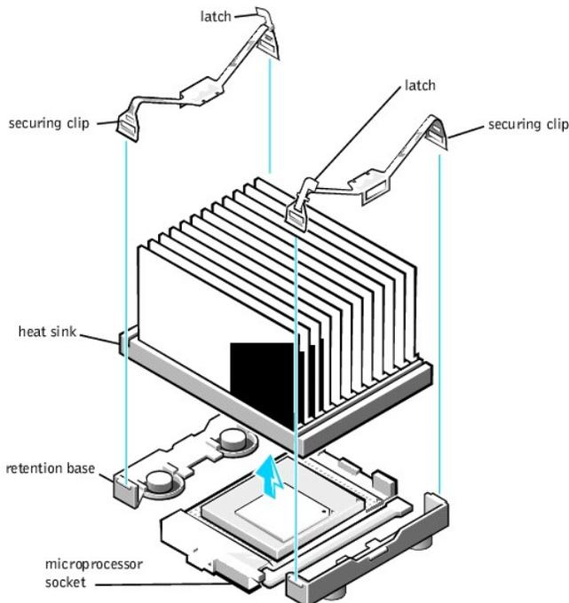
3. Remove the microprocessor from its connector.
