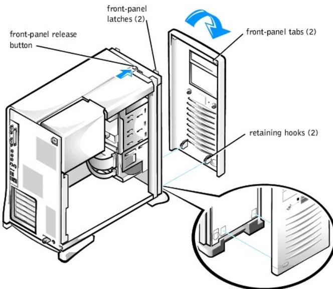
3. While pressing the front-panel release button, rotate the top of the panel outward, away from the chassis.
