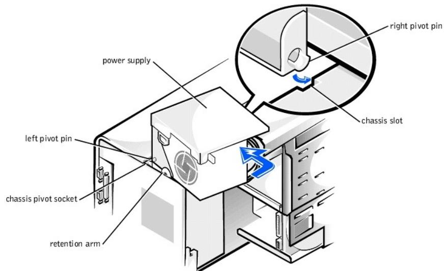
8. Lift the power supply away from the chassis.
