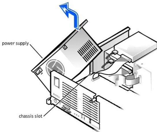
6. Lift the power supply away from the chassis.
