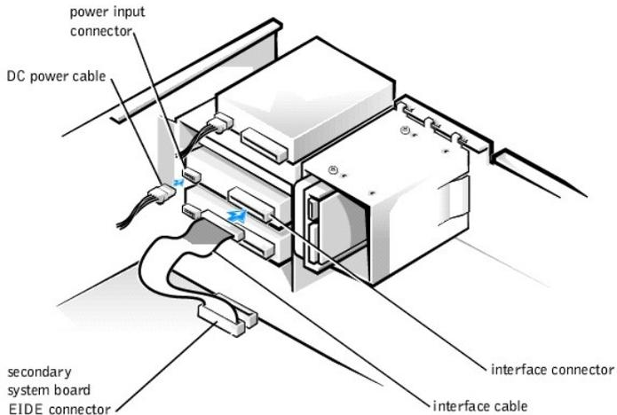
5. Ensure that all cables are firmly connected. Fold cables out of the way to provide airflow for the fan and cooling vents.
