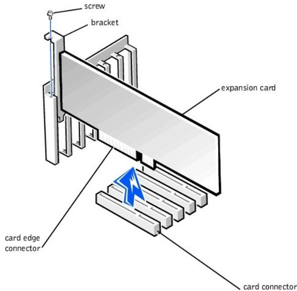
➡ **NOTICE:** An AGP Pro50 card may use multiple screws on its bracket. Install all screws on the expansion card's bracket.
