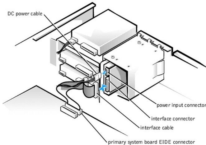
6. Ensure that all cables are firmly connected. Fold cables out of the way to provide airflow for the fan and cooling vents.
