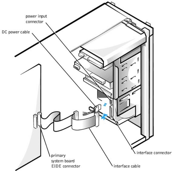
6. Ensure that all cables are firmly connected. Fold cables out of the way to provide airflow for the fan and cooling vents.
