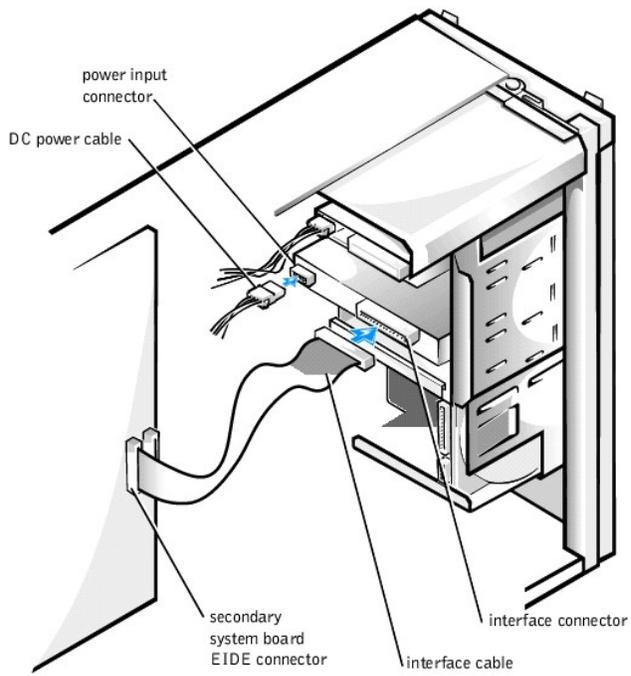
5. Ensure that all cables are firmly connected. Fold cables out of the way to provide airflow for the fan and cooling vents.
