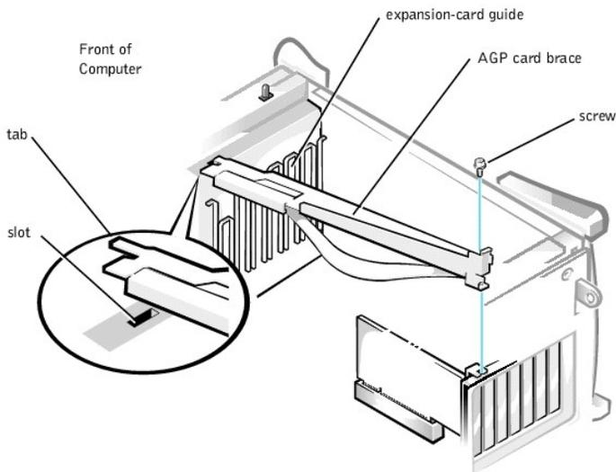
4. Rotate the brace up until it disengages from the card guide at the front of the chassis. Then lift the brace away from the chassis.
