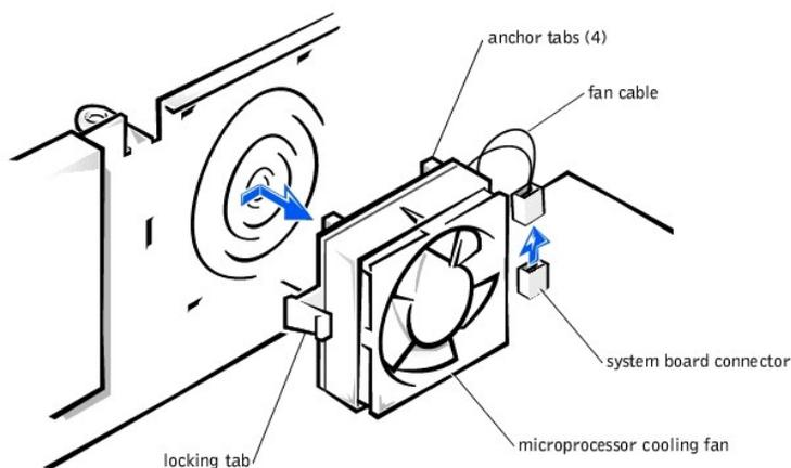
6. Lift the fan out of the chassis.
