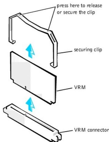
4. Grasp the VRM by its top corners, and ease it out of its connector.
